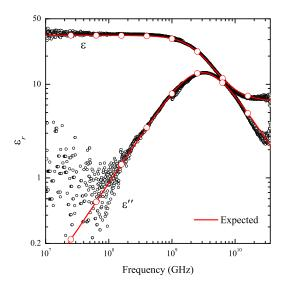
Figure 6: The real and imaginary parts of  $\varepsilon_r$  of a 99.9% sample of methyl alcohol at 28°C from 10 MHz to 36 GHz. The solid curves show the expected permittivity and were generated using Eq. 9 with parameters obtained from Ref. [3].
