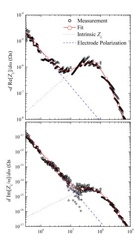
Figure 8: Logarithmic plots of  $-d\text{Re}\left[Z_L\right]/d\omega$  (top) and  $d\text{Im}\left[Z_L/\omega\right]/d\omega$  (bottom) as a function of frequency for the aqueous NaCl solution. The low-frequency power law behaviors can be used to parameterize  $R_p$  and  $C_p$ . The solid curves are fits to Eqs. 31 and 32. The dashed lines highlight the electrode polarization contributions.
