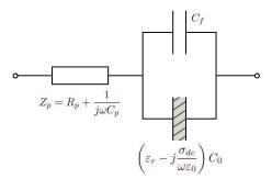
Figure 7: Electrode polarization effects can be modeled with a complex impedance  $Z_p$  in series with the intrinsic impedance due to the submerged tip of the open-ended coaxial probe. The MUT, of complex relative permittivity  $\varepsilon_r$  and conductivity  $\sigma_{dc}$ , is represented by the hatched region filling capacitor  $C_0$ .
