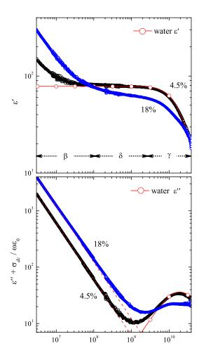
Figure 10: The real (top) and imaginary (bottom) components of  $\varepsilon_r - j\sigma_{dc}/\omega\varepsilon_0$  of WAS as a function of frequency from 3 MHz to 40 GHz. Samples with both 4.5% (black) and 18% (blue) solid concentrations were measured. The dashed lines have slope -1 and represent  $\sigma_{dc}/\omega\varepsilon_0$  contributions. The solid red curve is  $\varepsilon_r$  of pure water.
