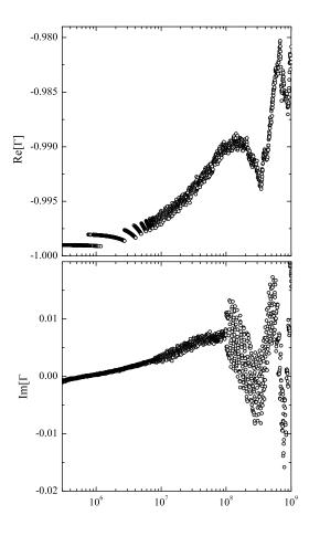
Figure 2: The real (top) and imaginary (bottom) components of  $\Gamma(\omega)$  of the short-circuited UT-141 coaxial probe as determined from the measured  $\rho_m(\omega)$  using Eq. 6 and the fitted value of  $\beta\ell$ . Note the very fine scales of the vertical axes. The step-like feature of Re[ $\Gamma$ ] at low frequency is due to a digitization of the VNA measurement of Re[ $\rho_m$ ].
